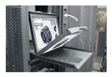
■ Flip up the LCD to a suitable angle.
