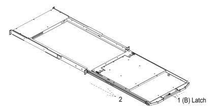
Step five Unlock Latch (B) to the left again to lift up LCD.
